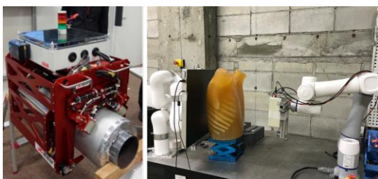
Fig. 2. (Left) A pipeline inspection robot equipped with a compact X-ray source for on-site non-destructive testing. (Right) A robotic X-ray CT system utilizing two robotic arms for precise positioning and scanning of complex objects.
