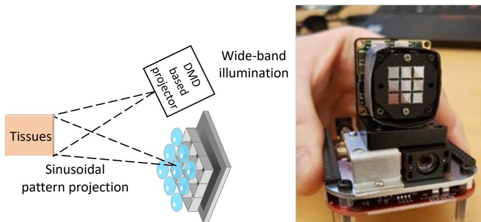
**Fig. 1.** Concept of compact SFDI device.
