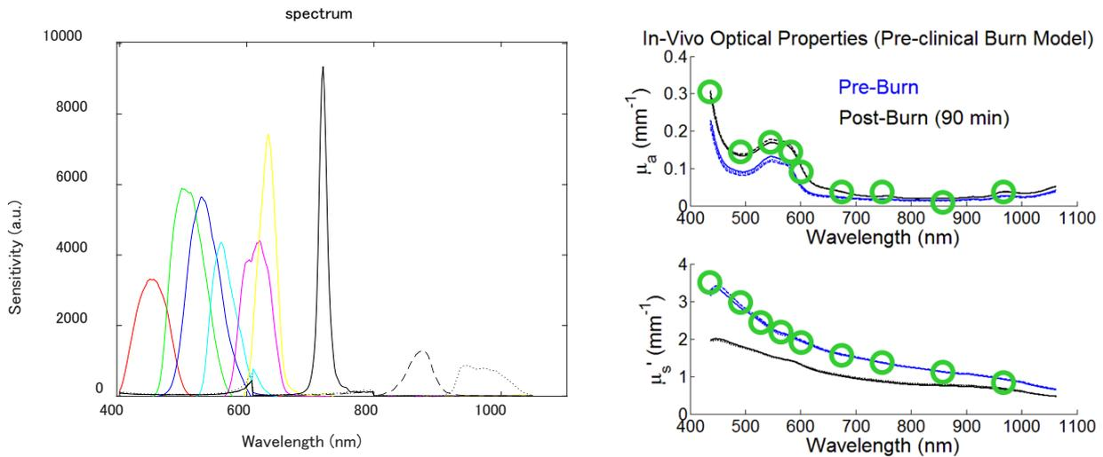
**Fig. 3.** Measured total spectral response of all 9 channels of the camera and the emulated spectral measurements from burn tissue response (derived from SFDS measurements in the previous preclinical study)
