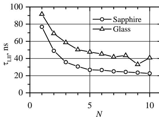
Fig.5. LII decay time as a function of the laser shot number in the sequence for carbon particles on glass and sapphire surfaces.
