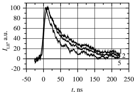
Fig.4. Typical LII oscillograms of carbon microparticles deposited on a glass surface by laser ablation technique.
