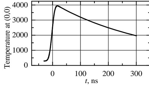
Fig.2. Calculated particle temperature history. Coordinates (0,0) correspond to the center of the particle's top surface.
