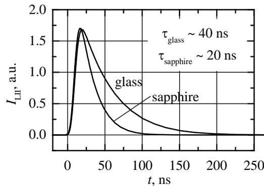
Fig.3. Calculated LII oscillograms for a carbon particle on a glass surface and on a sapphire surface.
