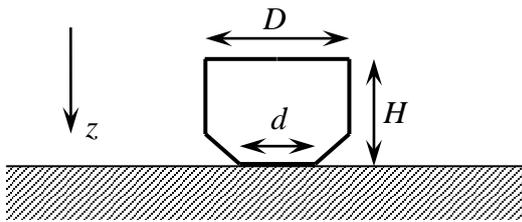
Fig.1. Carbon particle dimensions ( $D$  – diameter,  $H$  – height,  $d$  – particle-to-surface contact spot diameter).
