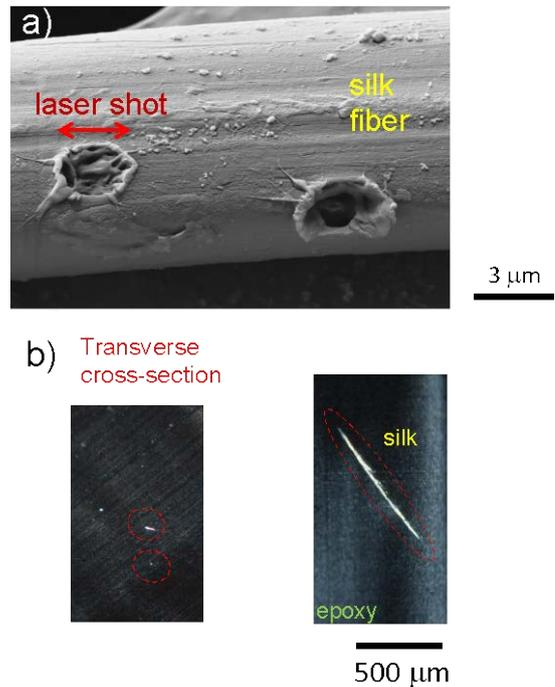
**Fig. 3.** Femtosecond laser fabrication of silk fibers embedded in a polymer matrix (a), transverse (left) and longitudinal (right) cross-section of the fiber showing the extent of laser fabricated areas.
