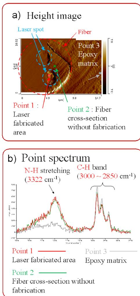
**Fig. 4.** Selection of laser-irradiated and pristine areas on cross-section of silk fiber (a), infra-red absorption spectra measured in these areas, and a similar spectrum measured in the epoxy matrix (b).
