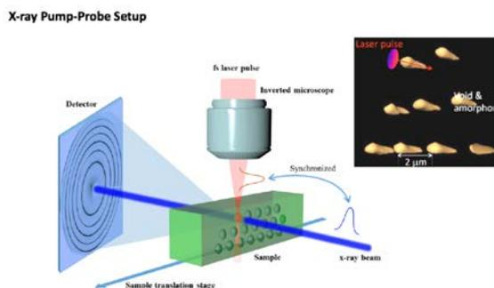
**Fig. 1.** Time-resolved XRD experiment. X-ray pulse delayed by a variable time with respect to the laser pulse probes transient state of WDM created by the latter. Depending on the delay, different XRD patterns reflecting the transient state can be registered. To ensure that fresh regions of the material are always probed, the sample is translated by a sufficient distance between two subsequent laser shots.
