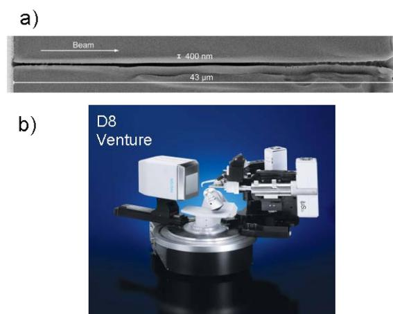
**Fig. 2.** Cross-sectional view of glass fabricated by Bessel beam illustrates the increased photomodified volume (a), the increased volume can possibly be characterized by the available laboratory X-ray diffraction equipment.
