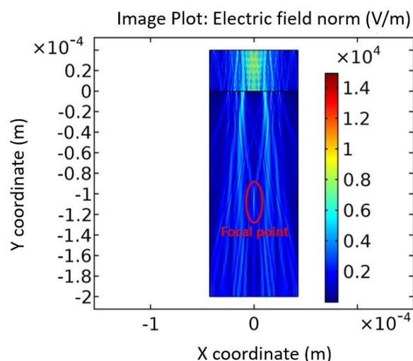
Fig. 2: Simulation of the modulus of the electric field in the region of the zone plate, showing focusing in the downstream region.
