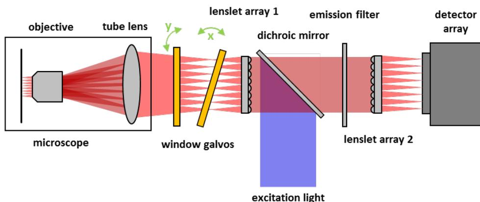
**Fig. 2:** Experimental setup of multifocal confocal scanning microscope.
