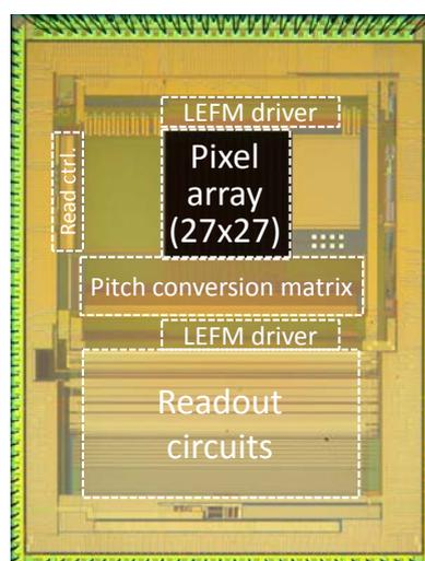
**Fig. 3:** Microphotograph of a prototype time-resolving CMOS image sensor.
