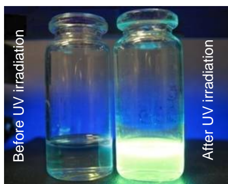
Fig. 5. Organic photosensitive chromone-based compound becomes light-emitting material after ultraviolet irradiation.
