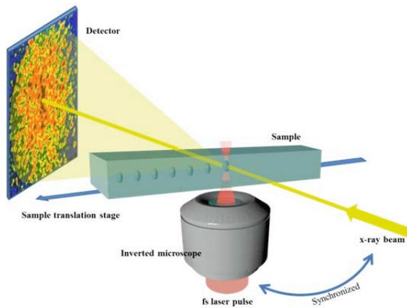
**Fig. 1.** Time-resolved XRD experiment. X-ray pulse delayed by a variable time with respect to the laser pulse probes transient state of WDM created by the latter. Depending on the delay, different XRD patterns reflecting the transient state can be registered. To ensure that fresh regions of the material are always probed, the sample is translated by a sufficient distance between two subsequent laser shots.
