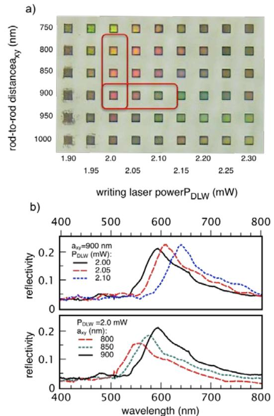
**Fig. 3.** Control of the structural color in 3D woodpile photonic crystals, (a) optical microscopy images of 3D woodpile PhC structures with different lattice periods fabricated at different exposure levels exhibit different colors in reflectance, (b) visible reflectivity spectra of these structures exhibit the corresponding spectral variations.
