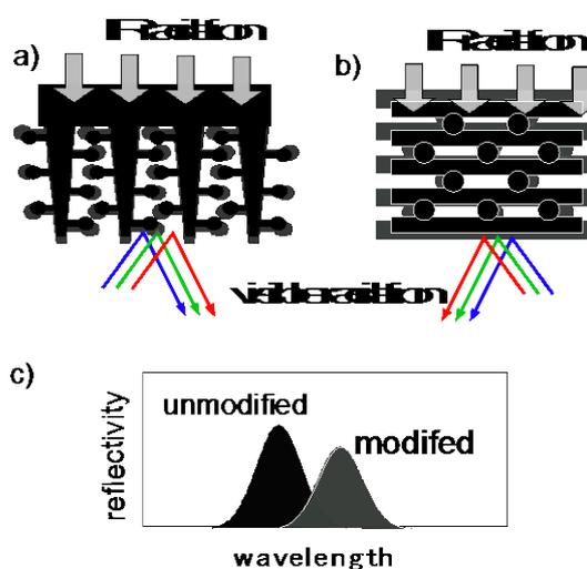
**Fig. 1.** IR sensitivity mechanism in natural and artificial in PhCs: (a) in natural *Morpho* butterfly wing, (b) in artificial 3D PhC structure, (c) modification of visible optical reflectivity of the PhC due to IR irradiation.
