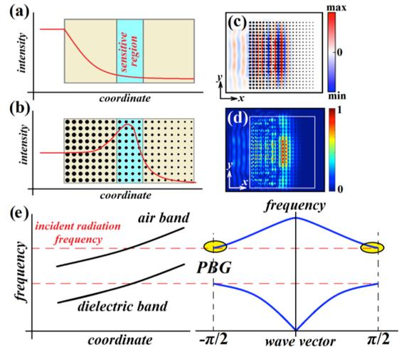
**Fig. 1.** Physical principles of optical field enhancement using ChPhC structures, (a) typical layout of a photodetector, (b) formation of field intensity peak within the structure, (c,d) numerically simulated intensity distribution inside the ChPhC structure, (e) spatial variation of photonic band gap frequency along the ChPhC structure (left), and local photonic band diagram at a certain depth, with slow-light regions emphasized by ovals (right).
